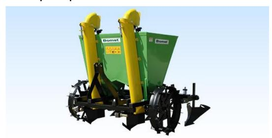
Potato planter is two-row planter mounted on the three point suspension system of tractor. The planter is mounted on the tractor with three point suspension system, **CAT 2**. During single cycle all the activities concerning with potato planting are performed (it makes furrows, automatically seeds the potatoes and ridges the seeded plants with soil).
