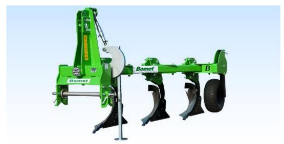
One-beam ploughs of U030 series are perfect for small and medium-sized farms in all soil conditions with tractors from 40 kM to 95 kM. The ploughs are intended for performing middle deep ploughing, on flat fields, slopes and hills on all types of soil. Spacing of bodies on the frame equaling 80 cm and clearance under the frame equaling 78 cm allows for unconstrained operation on fields with post-harvest residues.
